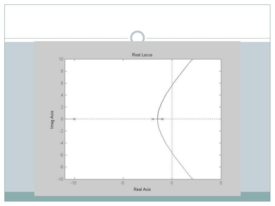
• The two complex branches of the root locus go unstable for values of K greater than 391. To allow for a larger range of stable gain values, we add the feedback path lead-lag compensator that places two zeros to the left of the pole at 2.
