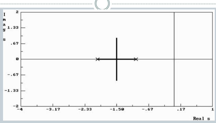
• We add a forward-path compensator that will place a pole and zero to the left of the two open-loop poles. The root locus is attracted to the compensator zero at s=-5.
