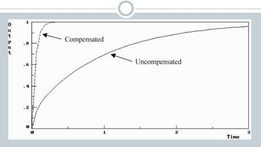
Time response characteristics with and without the lead compensator
